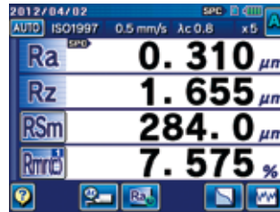
4-parameter display: multiple parameter measurement results
